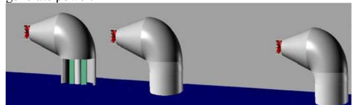
Fig. 1. Schematic representation of an array of concentric OWC devices
