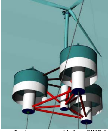
Fig.2. Multi-purpose floating structure with three OWC devices and a W/T (image below water surface)
