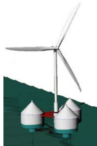
Fig.1. Multi-purpose floating structure with three OWC devices and a W/T (image above water surface)
