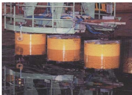
Fig. 3 Physical model of three OWC devices open to the atmosphere placed in a row
